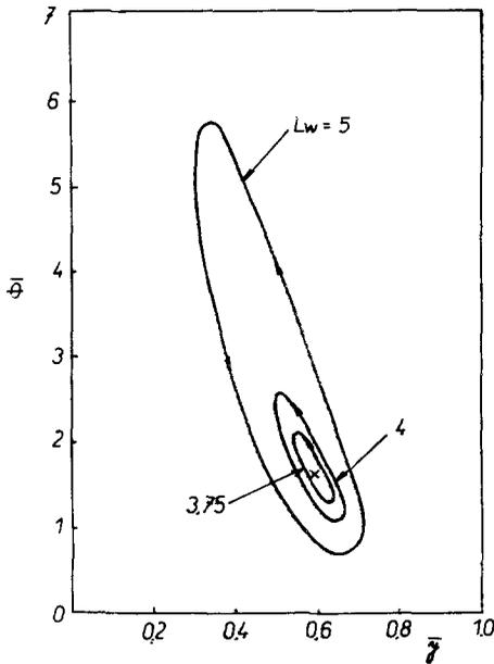
FIG. 10. The influence of  $Lw$  upon limit cycles.  $n = 1$ ;  $\gamma = 20$ ;  $\beta = 0.2$ ;  $\delta = 9$ ;  $a = 2$ .
